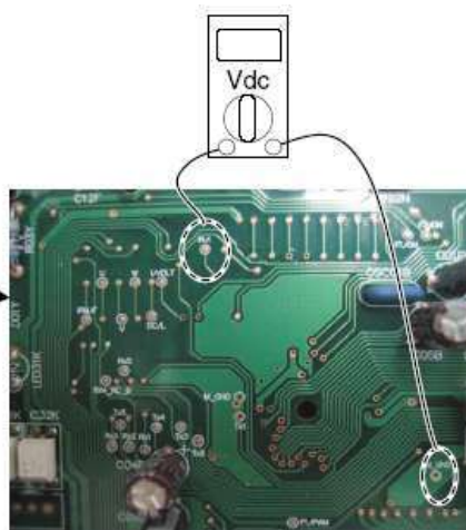
< CT Sensing Check Point >
